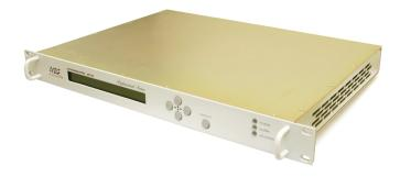
The receiver control interfaces are the front panel display, the local RS232 serial port (supporting CLI – control line interface) and the 10/100 Base-T Ethernet port (protocols supported: WEB, Telnet and SNMP).
